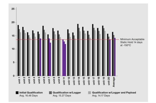
Temperature hold is affected by the thermal mass of the shipping device, which is also affected by other elements of the shipping configuration, such as data logger, rack, baffles, packaging, and the product. To get a true understanding of the expected performance of a dry shipper it must be validated with all elements in place.
